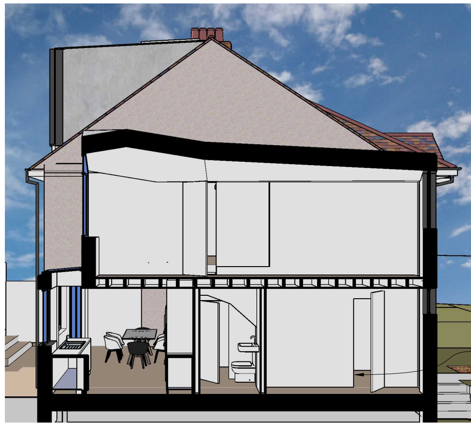
Section view through garage extension
